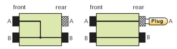
Allows: 1 output to feed 2 inputs Upper (A) and lower (B) channel separated
