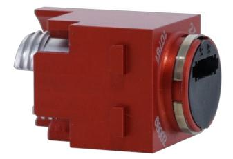
Benefiting from the expanded beam technology and the precision optical alignment the system creates high immunity against dust, mud, liquids and other contaminations. The FIBERFOX foxBRID module converts a standardized LC Patch cable into an expanded beam solution. It acts as a "feed-through" and fits into industrial standard shells.
