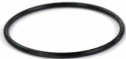
figure 9: O-ring after 5.000 mating cycles
