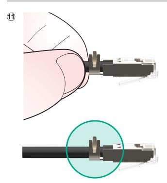
In the case of using shielded cable crimp shield to connector.
