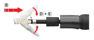
Position the chuck onto the RJ45.
