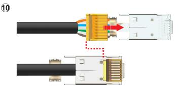
Insert wires and wire manager into RJ 45 plug and push fully forward.
