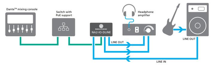
Using the Dante<sup>™</sup> adapter, the two applications described above can also be operated simultaneously (= mixed mode).
