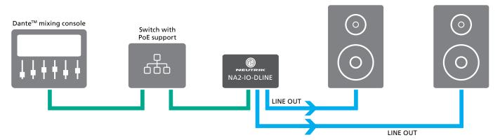
Loudspeakers and amplifiers that do not support  $Dante^{TM}$  can be connected to a  $Dante^{TM}$  network using the  $Dante^{TM}$  adapter.
