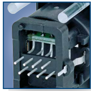
Vertical PCB with lightpipes
